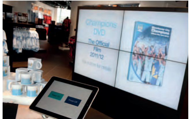
An AMX app transforms the iPad into a fully functional wireless touchpanel for controlling the Inspired XPert signage platform
